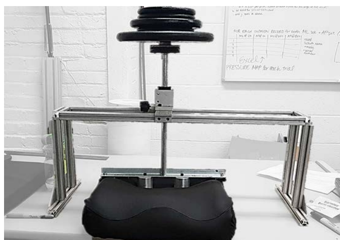
Figure 3. Test fixture used for CMS coding verification for wheelchair seat cushions
