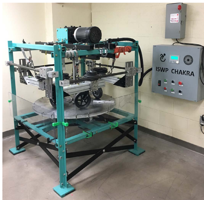
Figure 1. Caster testing system
