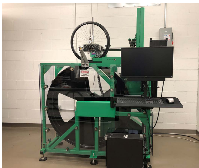
Figure 2. Wheel rolling resistance test system
