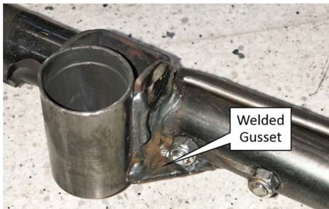
Figure 4. Improved GEN_2 with welded gusset.
