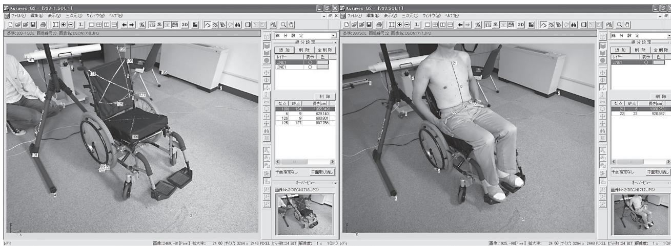
Figure 2 The three-dimensional measurement method uses two cameras and software to process the images
