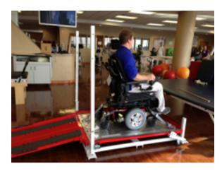
The training ramp has been rolled out of its storage place underneath a mat table. The platform elevates with a small electric motor allowing the ramp to assume several slopes. The top surface is a Q'Straint training platform with adjustable, WC18 compliant securement straps and hook end fittings.
