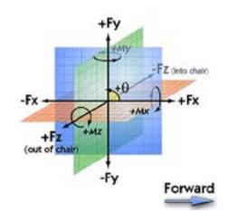
Figure 1. Force vectors and moments of the SmartWheel (SmartWheel Users Guide, 2010)
