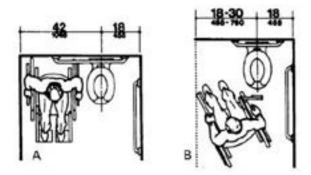
Figure 1. Two different wheelchair setups for toilet transfers suggested by the Access Board: wheelchair setup at the side (A) and in front of a toilet (B) ("Americans with Disabilities Act (ADA) - Accessibility Guidelines for Buildings and Facilities,")
