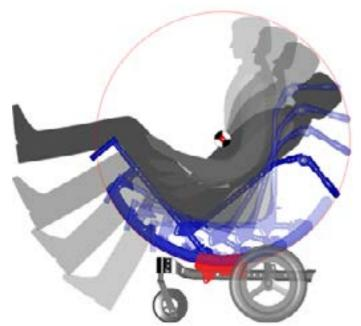
Graphic 2 is an example of a tilt in space wheelchair that tilts around the client's center of gravity.
