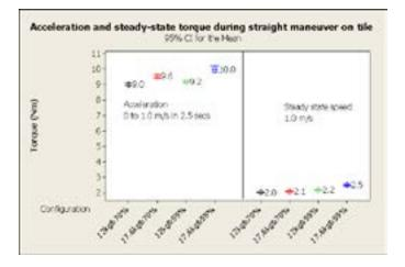
**Figure 1** also illustrates the relative influence of mass and mass distribution. During acceleration, mass has a greater influence, evidenced by the greater torques required of the 17.6 kg chairs. This difference, however, is not present during steady state velocity during a straight maneuver. Since inertia is not a major influence during this phase, the frictional losses are reflected in these torque measurements.
