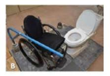
Figure 3. The orientation of the toilet in side (A) and front (B) setups in our transfer station. For the side setup, both of the wheelchair and toilet faced forward, and there was a small angle between the wheelchair and toilet. In the front setup, the toilet was rotated 90 degree and faced to the wheelchair. There was a large angle (larger than 90 degree) between the wheelchair and toilet.
