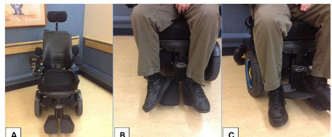
*"A three photo series of a front wheel-drive power wheelchair with center-mounted footplate by itself, showing a user sitting with externally rotated hips and foot eversion on the footplate, and showing the user's limb falling off the footplate and at risk for injury."*
