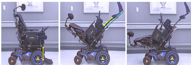
*"A three photo series of a front wheel-drive power wheelchair with markers showing the increased length of the center-mounted legrest between the knee joint and the footplate when changing position from fully upright to full tilt with legrests extended."*
